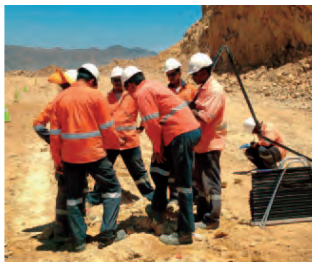
Sukari team examining a drill hole in readiness for explosives
