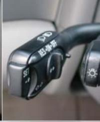
**BODY CONTROLS** HID-headlights Suspension Gear **Headlight Adjustment Speed Control** Steering **Traction Control** Wiper Control
