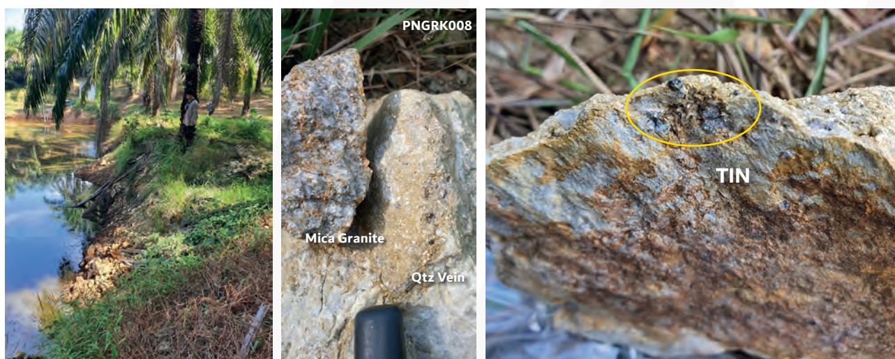
FIGURE 17: Phang Nga sample PNGRK008 from a water course cutting showing tin mineralisation
