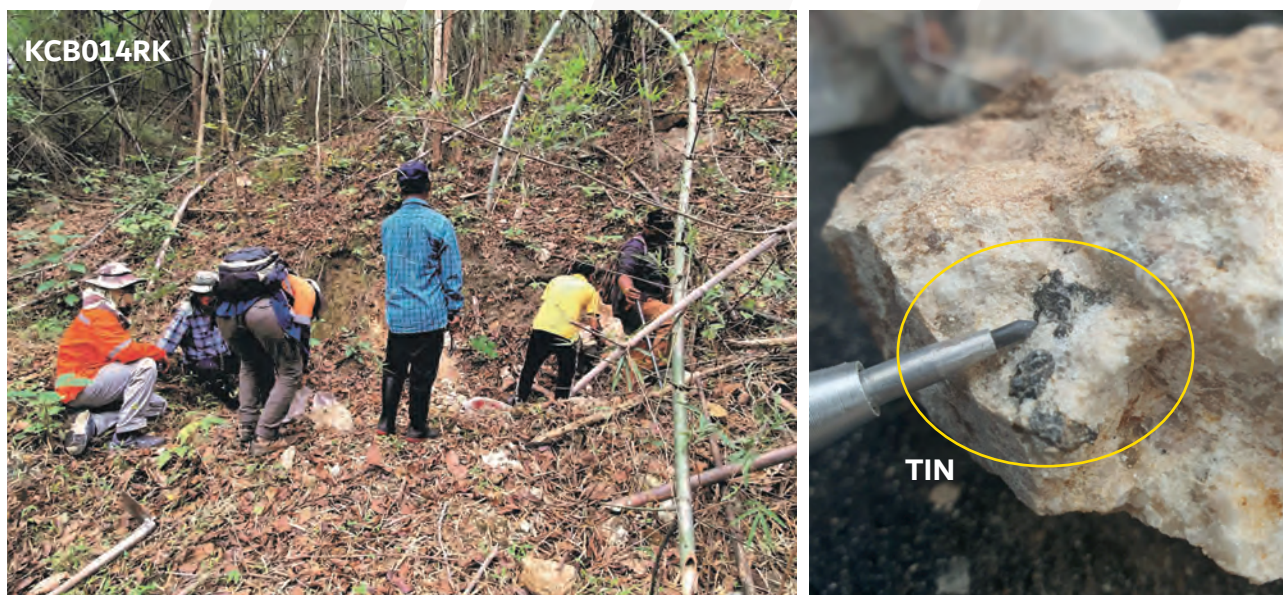
FIGURE 18: Kanchanaburi sample KCB014RK from outcropping pegmatite showing tin mineralisation. This pegmatite has been mapped over 2km strike, 600m wide and striking NW
