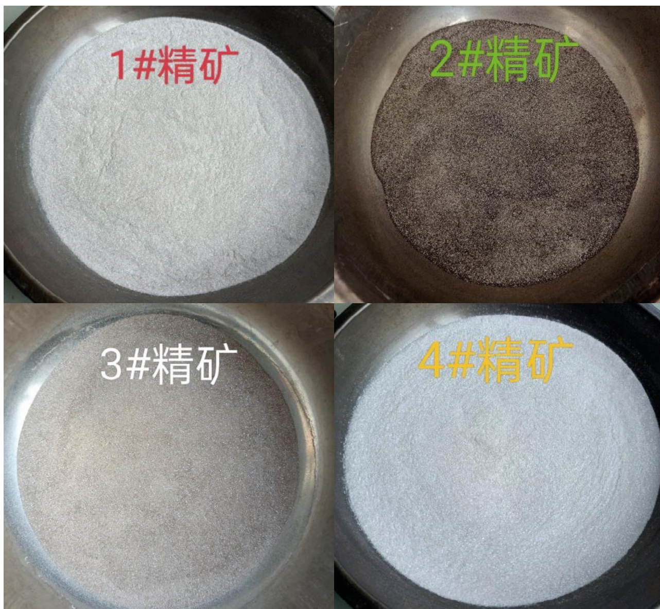
Photo Set: Matsa testwork flotation concentrate samples from left to right and top to bottom; lepidolite concentrate from Pink Panther, polyolithionite concentrate from Black Panther, polyolithionite concentrate from Spotted Panther & lepidolite concentrate from Rose Panther
