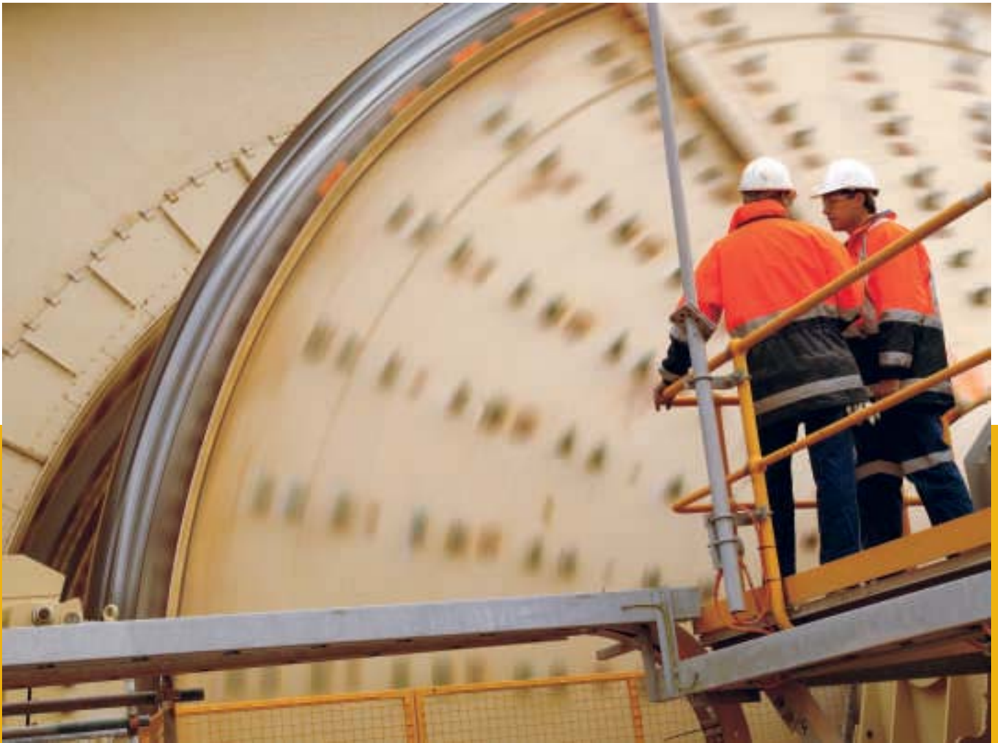
Above: Frank Reid and Sam Booth inspect the Semi-Autogenous Grinding Mill at Telfer.
