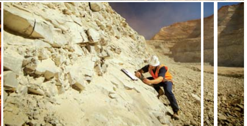
Page 29 top Diamond drilling at Cadia District. Page 29 lower left Contract driller at Cadia District. Page 29 lower right Glen Balog, Graduate Geotechnical Engineer measuring the orientation of the joint surface of the rock at the Telfer Mine.
