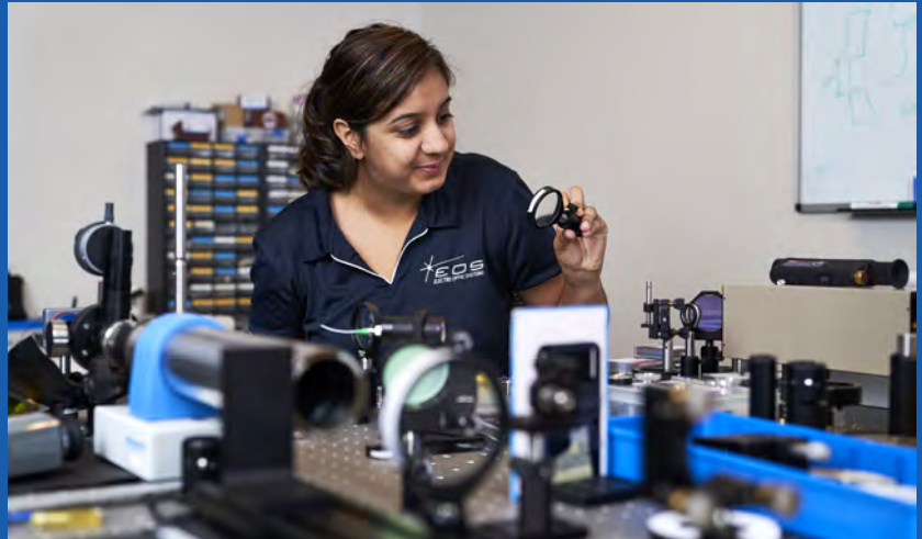
Namisha Chhabra inspects a lens that will help to align laser light into an EOS sensor
