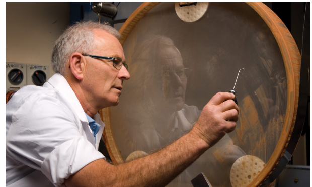
A KiwiStar Optics technician preparing for interferometric testing of an astronomical off axis parabola mirror
