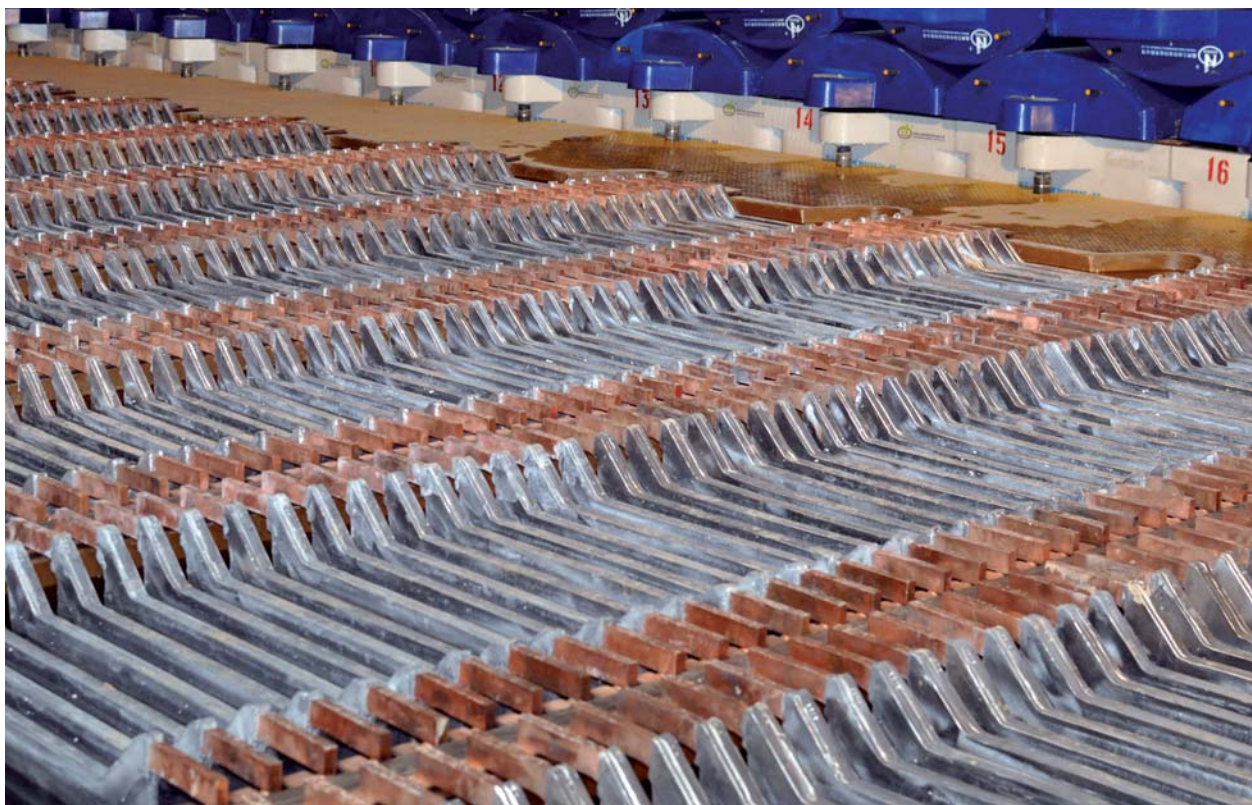
EW Cells loaded with anodes – EW plant Kounrad
