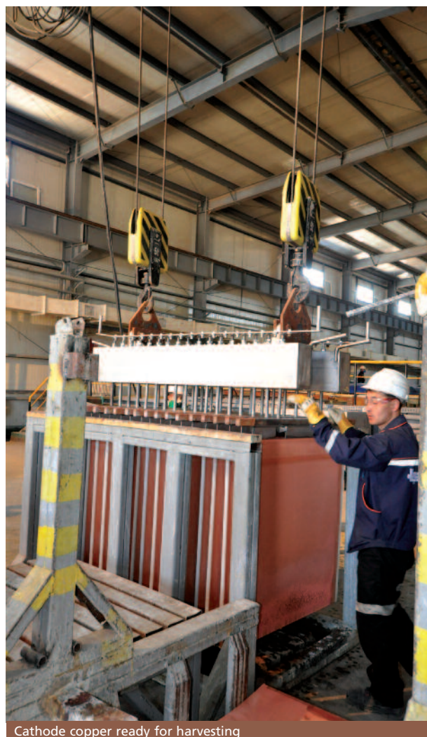
Cathode copper ready for harvesting
