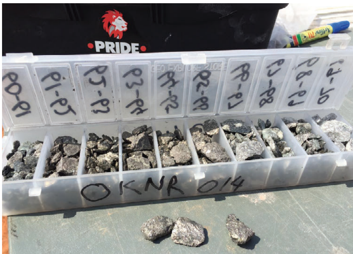
Figure 16: Massive sulphides in OKNR014 which returned 7m at 6.45% Zn and 0.43% Cu from 60m. (Note each divider shows chips from a 1m interval)
