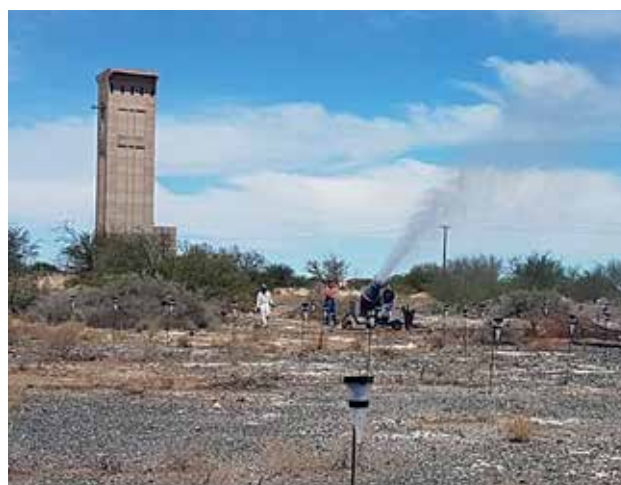
Feasibility study field trial of effectiveness of a 15kW evaporator at the Prieska Project. The planned pilot trials aim to test 75kW and 90kW units as the next phase of the program.
