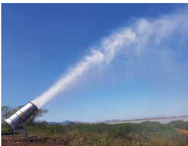
Feasibility study field trial of effectiveness of a 15kW evaporator at the Prieska Project. The planned pilot trials aim to test 75kW and 90kW units as the next phase of the program.
