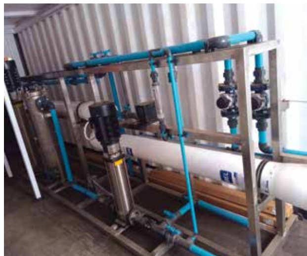
(Left) Water treatment pilot plant mobilisation. (Right) Commissioning the chemical treatment, filtration and reverse osmosis components of the pilot water treatment plant, setup to operate at 5m 3 /hr of feed water.
