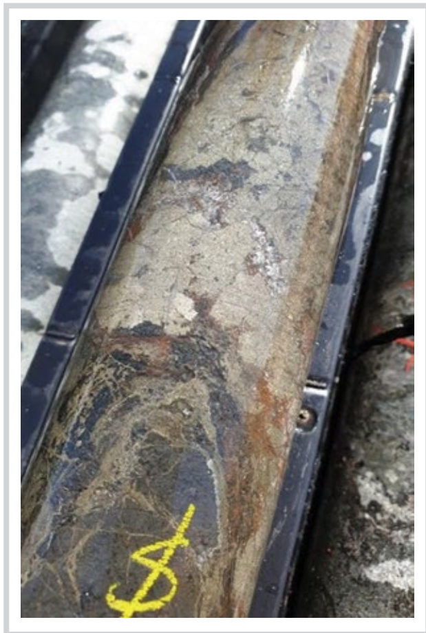
Figure 23: Semi-massive to massive pyrrhotite-pyrite vein at 331m down-hole depth in drill hole 19AFDD1008 drilled on the Hook 1 prospect.
