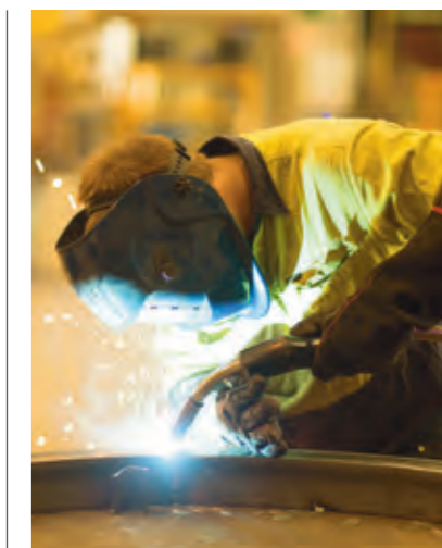
Above A Monadelphous boilermaker fabricating a valve pit flange for BHP Billiton's Olympic Dam borefield water supply pipeline, Roxby Downs, South Australia.
