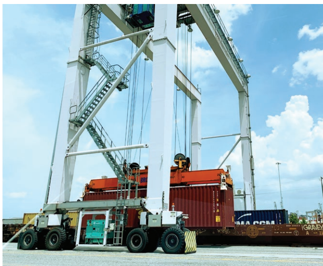
Figure 2. Container crane at Port of Savannah showing wheels on “runway”.
