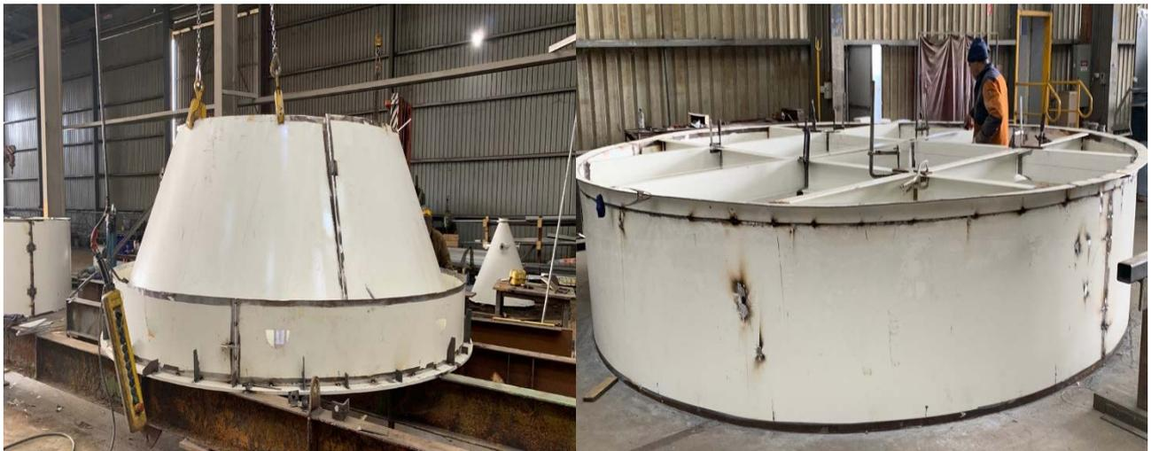
**Workshop Fabrication of Spray Roaster Reactor Shell and Oxide Bin**
