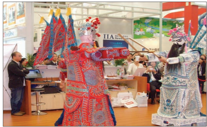
OPERA-SINGING ROBOTS – PSoC controls the eye movements of these robots, built by students at Shanghai Jiaotong University and showcased at the 2010 Shanghai World Expo.
