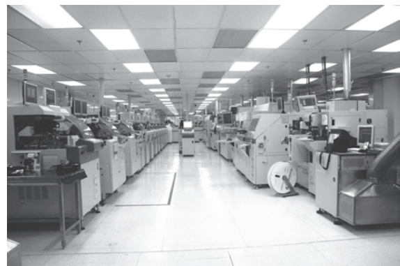
Figure 9. The Autoline in the picture above accepts wafers at the loading table on the left and moves them through die attach and wire bond to the large plastic molding machine at the far end of the line. On the return trip, the molded units are baked, laser-marked, sawed apart, electrically tested, QA tested and packaged—in the case of this Autoline, onto the tape-and-reel system on the right hand side. The Autoline also prints shipping labels, allowing the reels to be shipped directly. Each of our nine Autolines produces 3,600 to 10,000 units per hour, but requires only four technicians to operate. Since the wafers are assembled and tested without human intervention, the quality defect level on an Autoline is factors better than on a manual assembly line. During 2011, our assembly and test plant, Cypress Manila Ltd. (CML) will become an Autoline-only factory.
