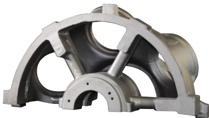
Pictured: Centre Case and Bearing Support castings for gas turbine
