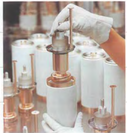
Manufacture of subassemblies for vacuum interruptors.
