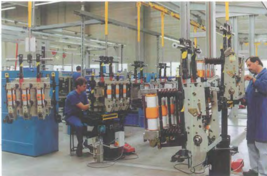
Production of vacuum high-performance power-breakers at the medium-voltage factory in Regensburg.
