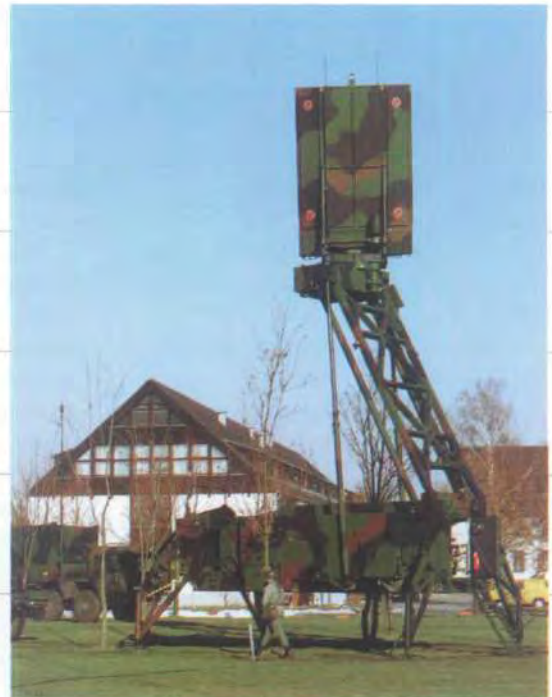
Mobile 3-dimensional radar system for the army anti-aircraft reconnaissance and command and control system.
