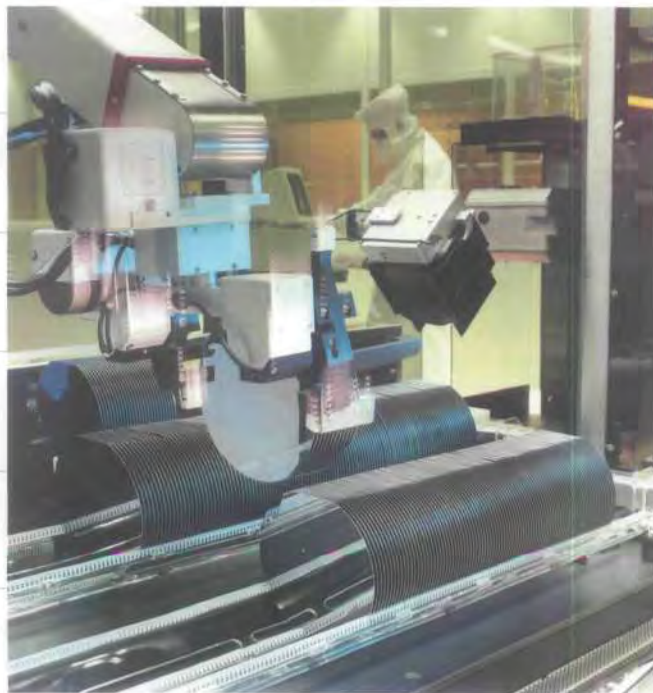
Flexible automated manufacturing of wafers in Heilbronn: robot charging station in diffusion.
