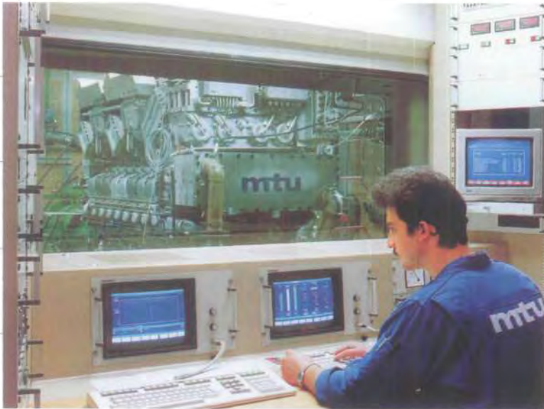
The new 16-cylinder V16-595 engine on the flexible computerized test stand.
