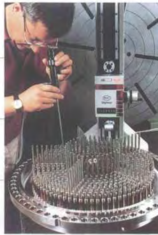
Inspection of the liquid hydrogen/-oxygen injection system for the Vulcain combustion chamber of the Ariane 5.
