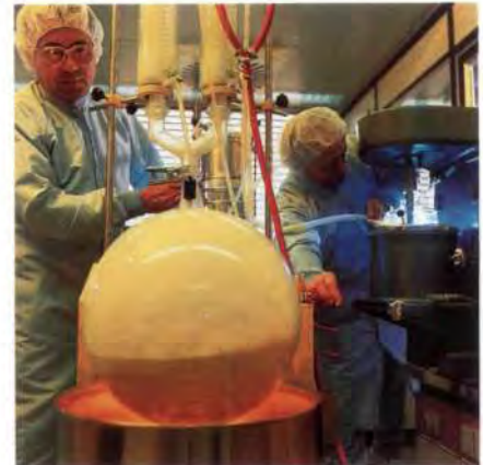
Silicon nitride powder mixture drying in the rotary evaporator – a preliminary stage in the manufacture of sintered ceramic parts for the automotive industry.
