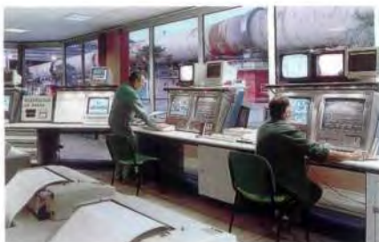
In the field of process automation, minimal primary energy consumption and operating effort plus optimized logistics are the principal market requirements. These requirements are met at the pilot facility in France where the Geamatics B central process control system controls and monitors cement production.
