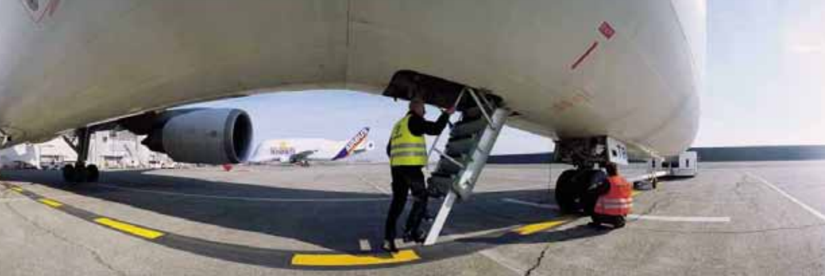
The Airbus A300-600 ST "Beluga" transport aircraft ferries large components from the European Airbus partners to the final assembly locations in Toulouse and Hamburg
