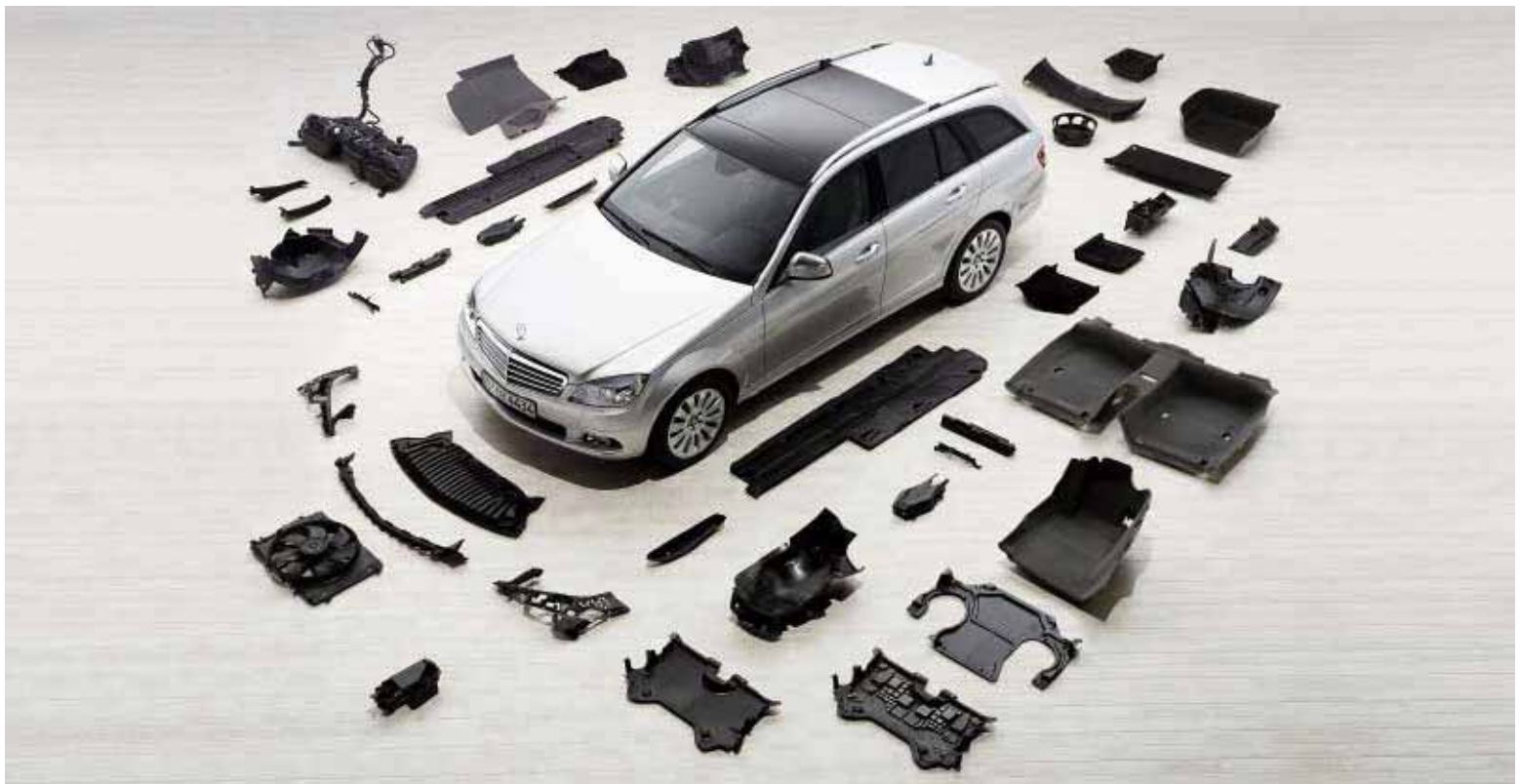
Mercedes-Benz C-Class station wagon with environmental certification: 39 components have been approved for recycled plastics, 32 components are made of renewable raw materials.
