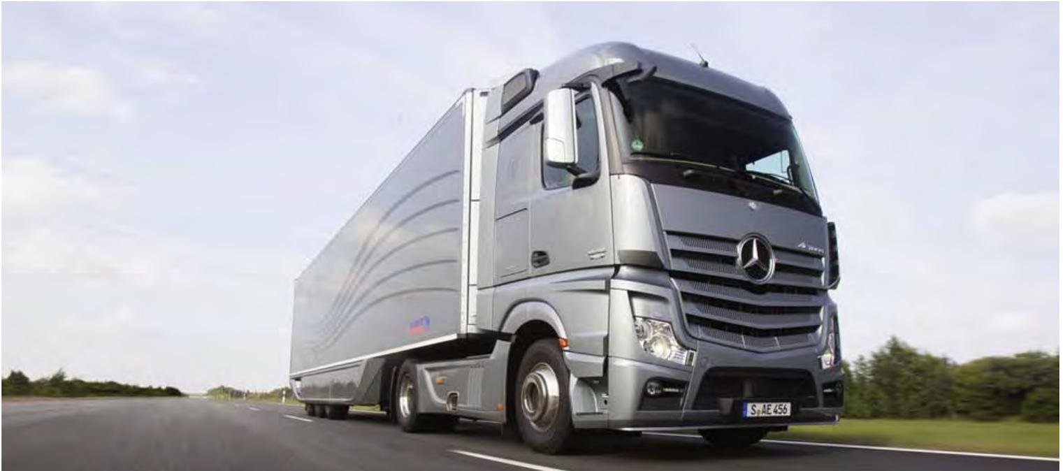
The Aerodynamics Trailer saves about 2,000 liters of diesel per semi-trailer truck each year while reducing CO<sub>2</sub> emissions by five tons.
