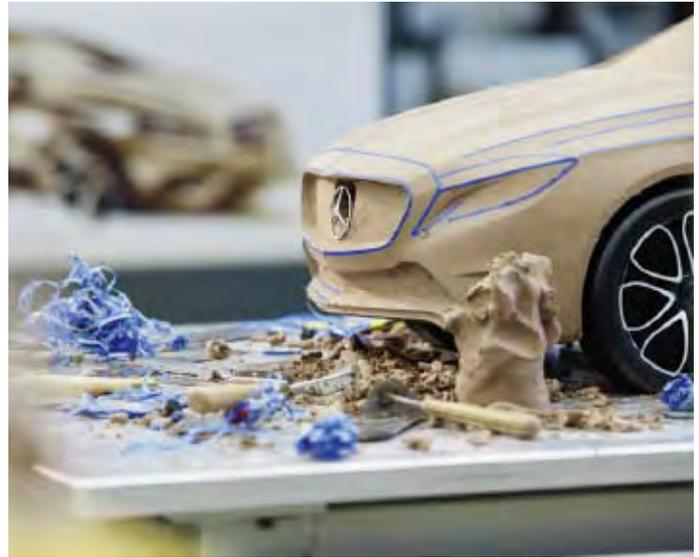
The unique sculptural quality of the new A-Class can be seen in its characteristic lines, well-defined edges, and taut surfaces. These fascinating shapes were initially handmade in clay.
