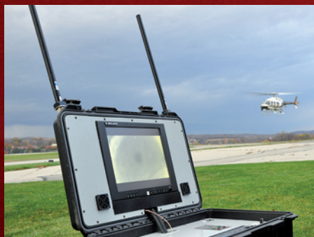
IMT's ruggedized COFDM 6-way diversity portable receiver/monitor.
