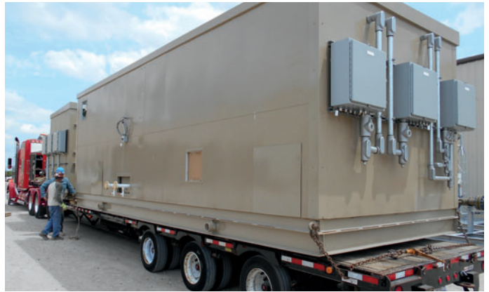
Climate controlled enclosures provide custody transfer measurement, sampling, analysis, and injection systems for Bakken region pipelines.
