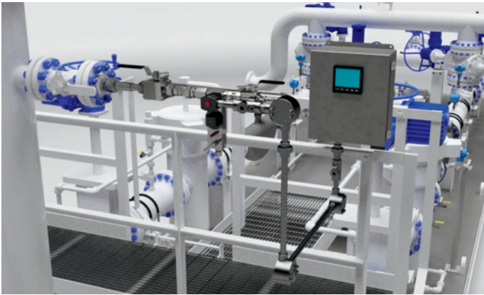
Oil and gas SMART Sampler unit taken from R&D into test application using advanced 3D design software.
