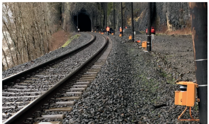
A new LIDAR-based monitoring system uses optical heads mounted to an existing break-wire fence to detect if an object is on the track and determine its size and location for risk assessment and safety.
