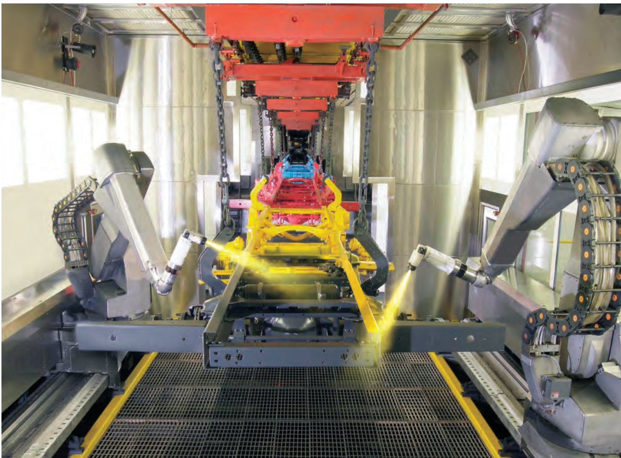
A world first in the commercial vehicle industry, Leyland added an innovative new robotic chassis paint facility in 2005 that helped boost capacity and achieve record production levels for DAF and Foden trucks.
