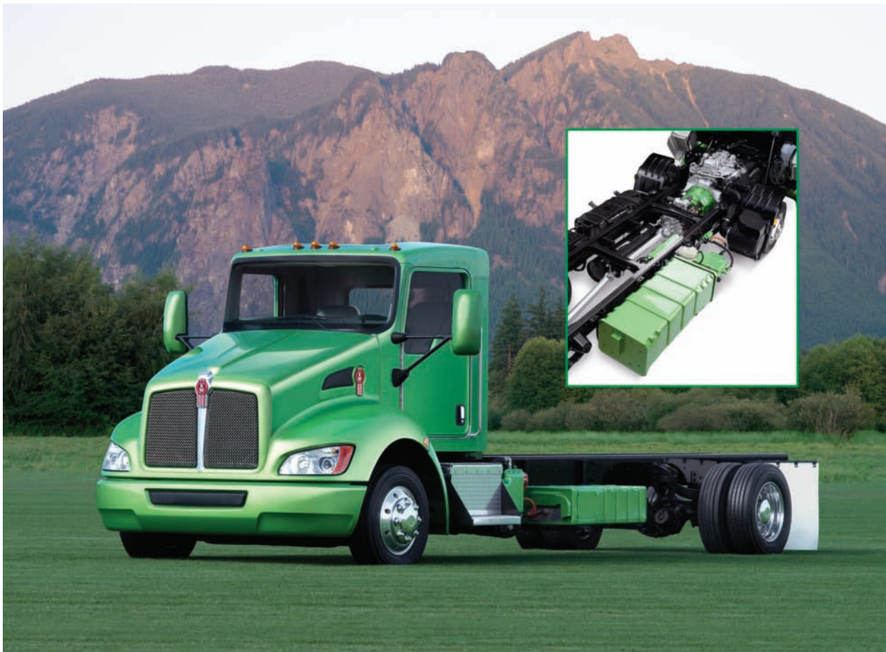
PACCAR Technical Centers are paving the industry in the development of hybrid-powered trucks. The Kenworth T270 medium-duty hybrid-electric truck has demonstrated fuel economy improvement of up to 30 percent in pickup and delivery applications.
