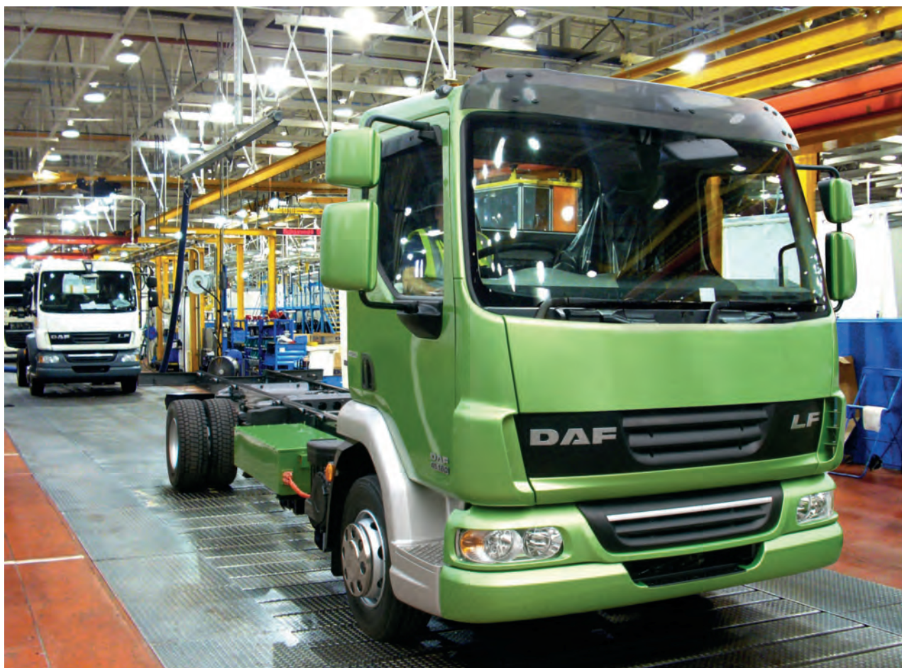
The award-winning DAF LF is now available in a Leyland-produced diesel-electric hybrid version that can improve fuel economy by as much as 30% over conventionally powered vehicles. This technology is designed for stop-and-go, urban pickup and delivery applications.
