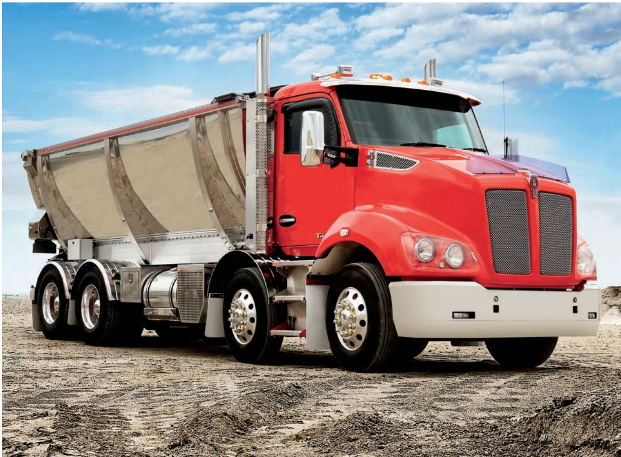
Kenworth trucks are designed and manufactured in Australia to perform in some of the most demanding applications in the world. The Kenworth T410 8x4 is powered by the PACCAR Integrated Powertrain, pairing the efficient PACCAR MX-13 engine with the smooth PACCAR TX-12 transmission.
