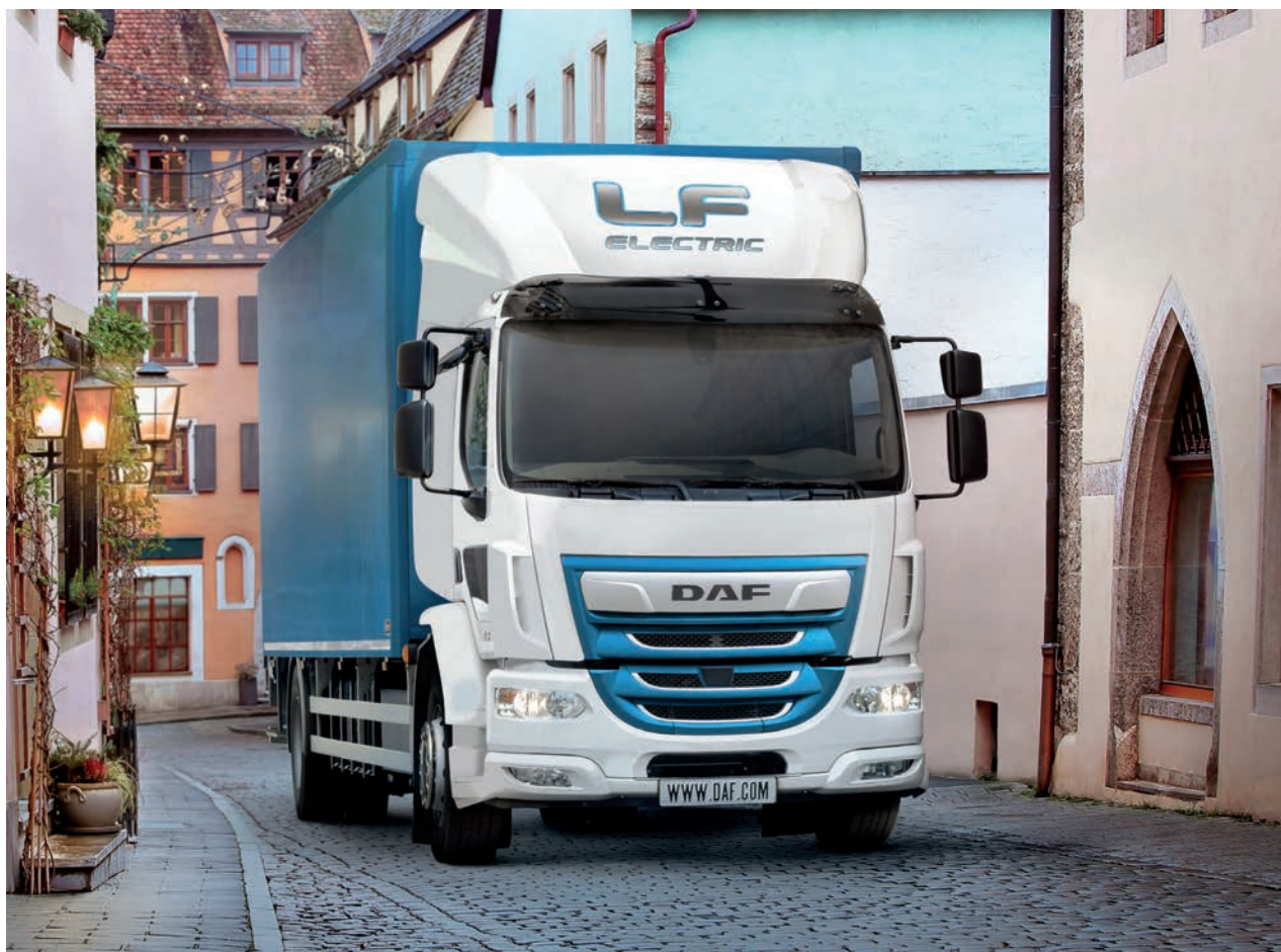
Leyland manufactures the full DAF product range of LF, CF, XF, XG and XG+ models for right- and left-hand drive markets. The LF Electric is suited for urban applications with a range of up to 175 miles using lithium iron phosphate (LFP) batteries that can be charged by AC or DC power.
