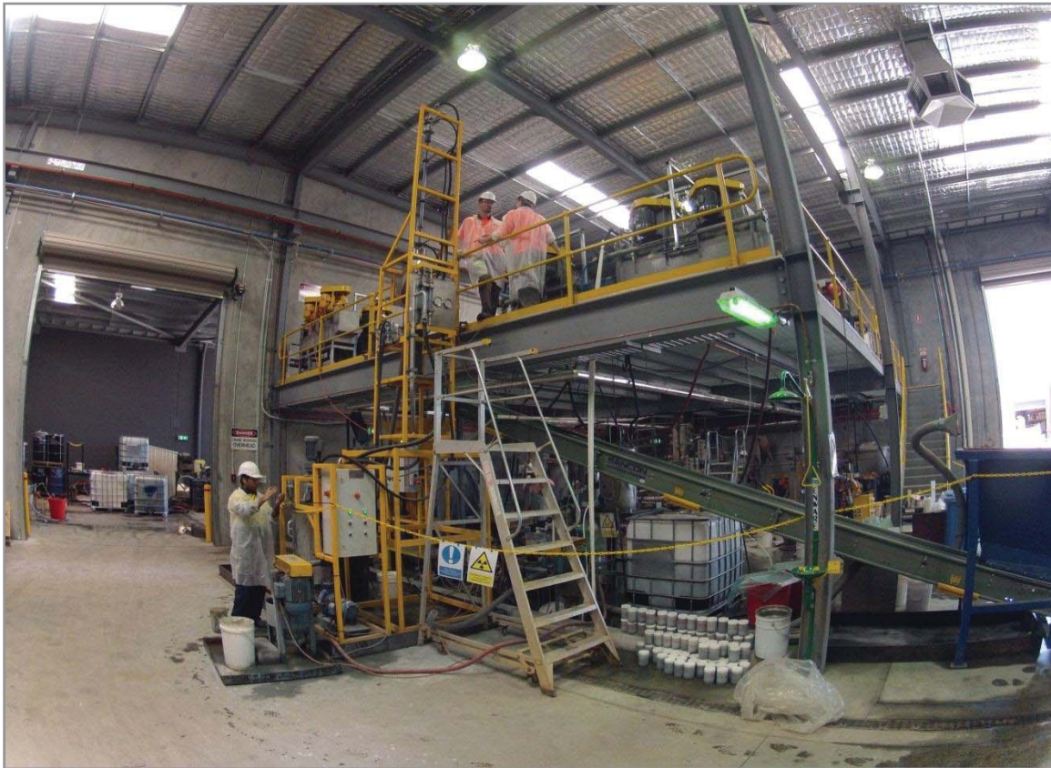
Overview of the pilot plant facilities with the Jameson Cell in the foreground.
