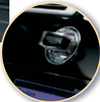
The Aston Martin vehicles use an electronic key fob and mating docking station developed by STRATTEC exclusively for Aston Martin.
