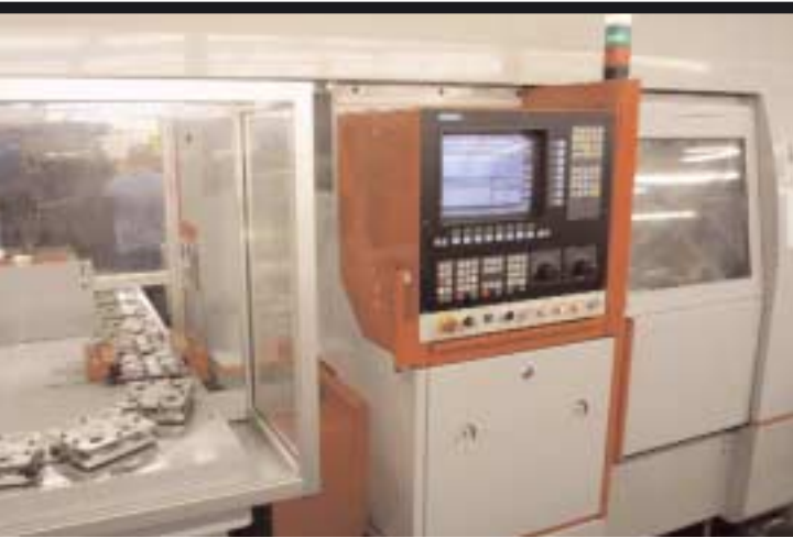
CNC Machine Center capable of lathe and mill work operations using both auto-bar and gantry loading methods at SMI
