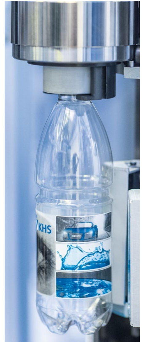
Printing direct onto PET bottles using low migration LED-cured UV ink with the Xaar-enabled Direct Print powered by KHS system
