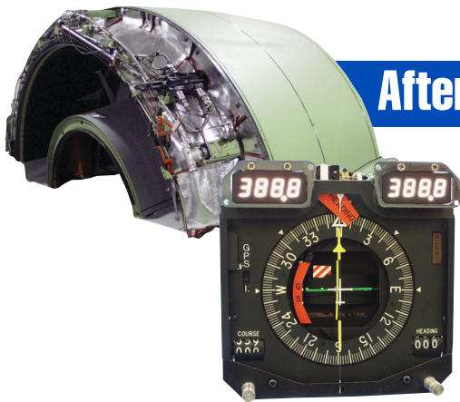
Above left: CF6-50 Fan reverser used on A300, B747, and DC10 passenger and cargo aircraft.
