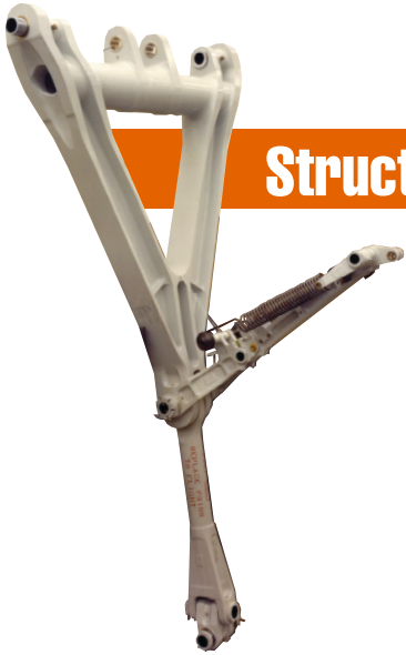
Above: Landing gear: drag strut assembly used on Boeing 767.
