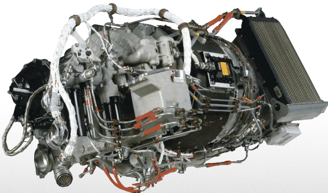
Above: GTCP-131-9 Series APU used on Boeing 737-700/800/900 and MD90 aircraft.
