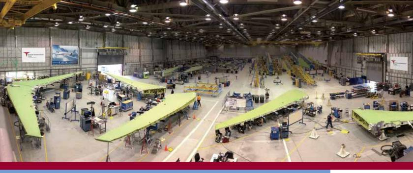
Triumph Aerostructures – Vought Aircraft Division – Tulsa assumed production of the Gulfstream G650 and G280 wing programs from Spirit Aerosystems. The addition of these programs positions Triumph as a leader in fully integrated wing design, engineering and production, and furthers its standing as a strategic Tier One Capable aerostructures supplier. Above, the Gulfstream G650 wing assembly is shown in production at the Tulsa manufacturing facility.
