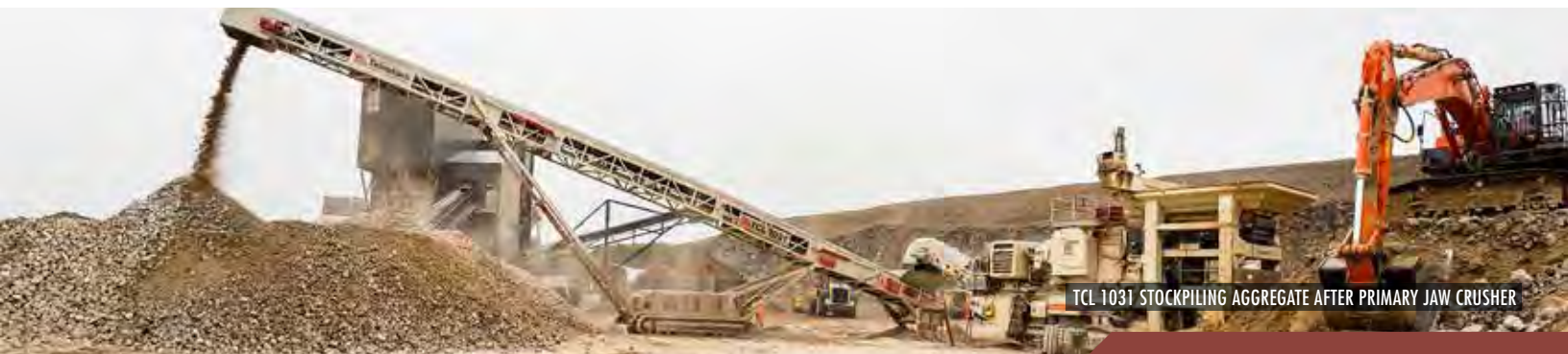
TITAN 450-4 BULK RECEPTION FEEDER AND TS650 RADIAL TELESCOPIC CONVEYOR
