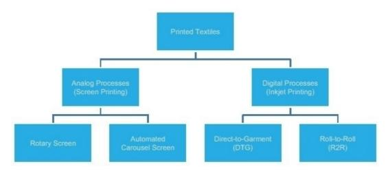
Screen printing is the most commonly used printing process for textiles. The two primary methods of screen printing are rotary screen printing and automated carousel screen printing.
