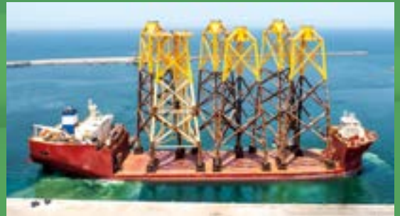
Jackets fabricated by Lamprell en route to the Moray East wind farm in the North Sea.
