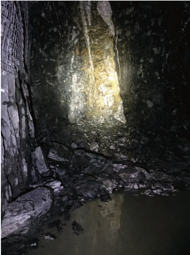
The High Grade Gold Vein at the Vivien Underground Mine showing extensive Sulphides
