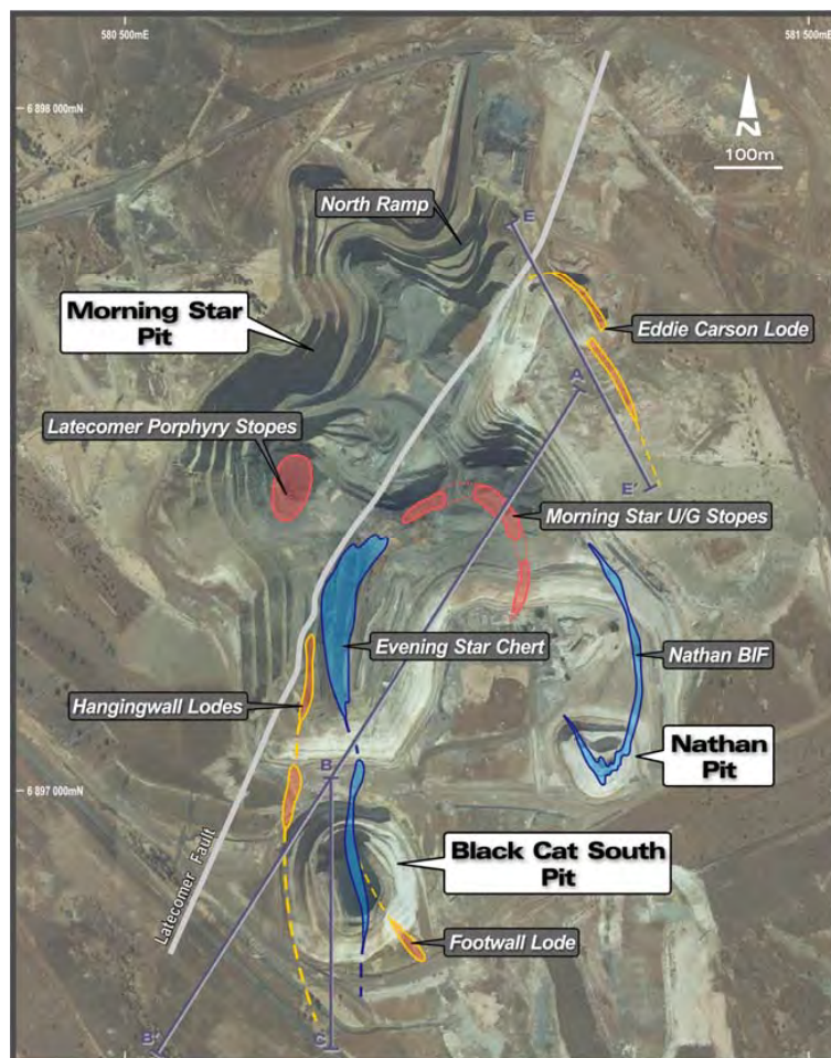
Figure 14: Morning Star pit plan view highlighting the Morning Star Deeps section A-B' and the saddle between Morning Star & Black Cat South pit B-C'
