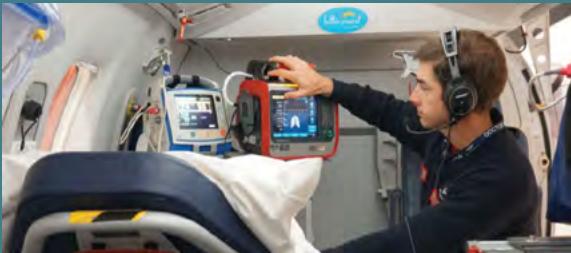
Hamilton T1 Ventilator installed into RFDS aircraft
