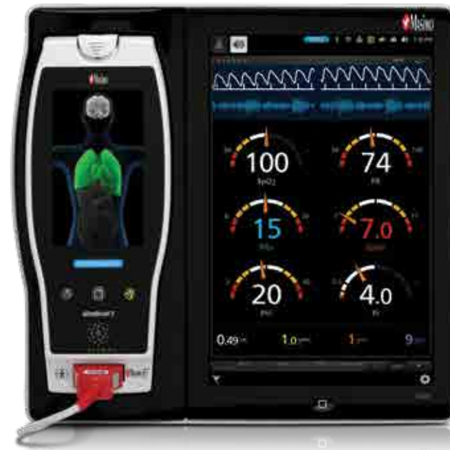
In Analog view, virtual gauges show measurement values in relation to alarm ranges.
