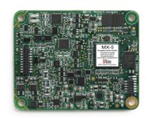
Signal processing apparatus for all Masimo technology platforms
