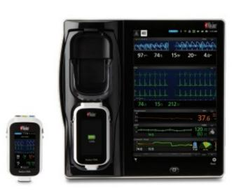
Use: • Radius VSM<sup>™</sup> monitors a wide range of measurements on a modular form; components can be customized based on each patient's monitoring needs
