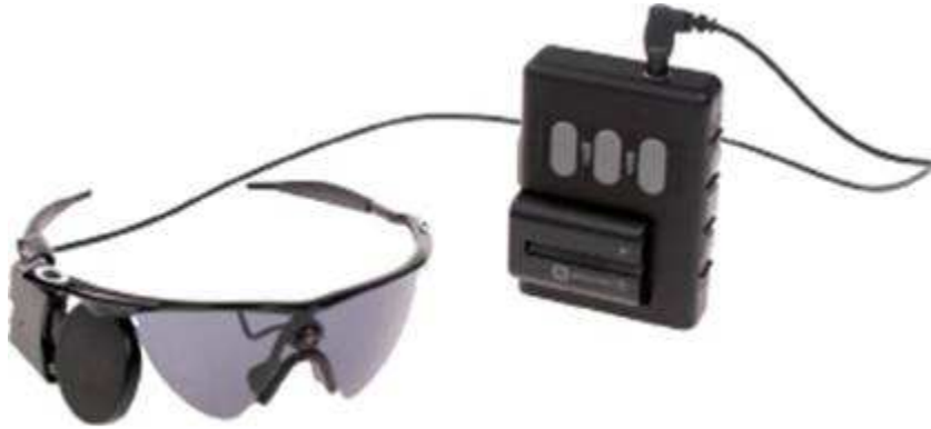
Figure 4: External Components of the Argus II System
