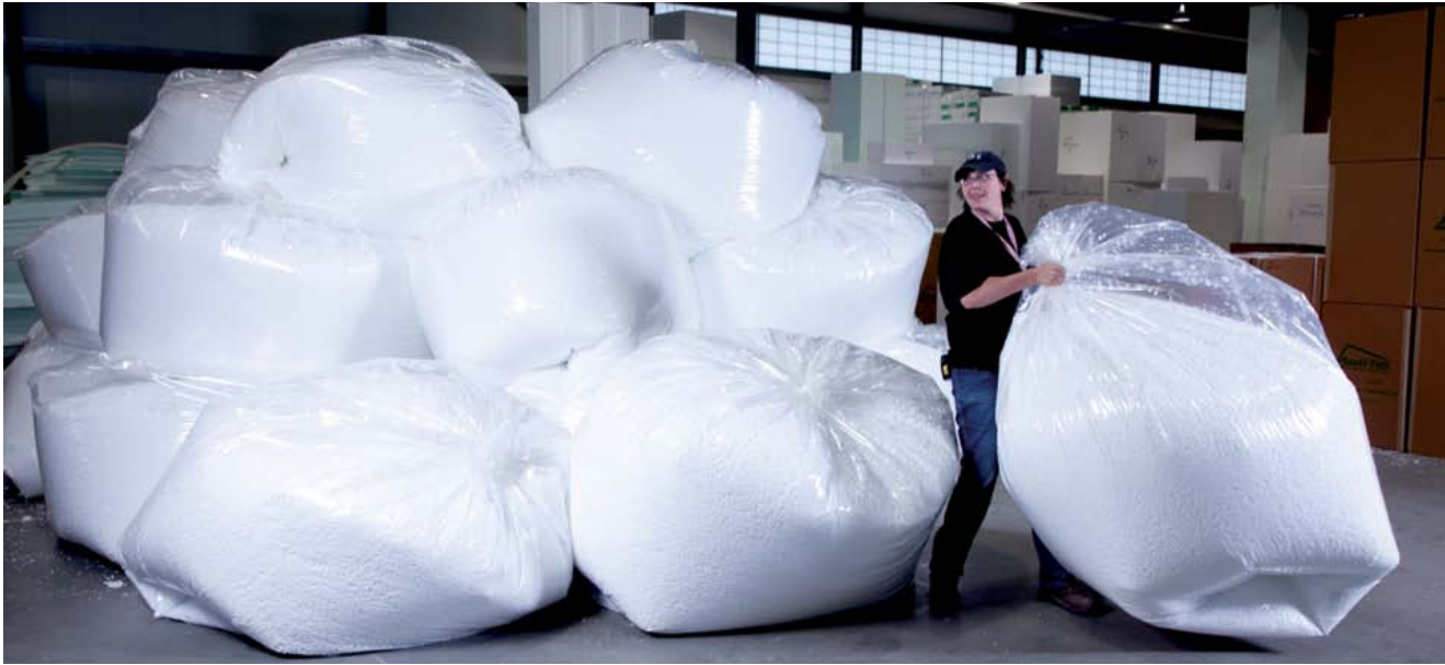
Reduce and Re-Use: A Block Molding plant employee stacks bags of regrind, an excess material that gets reground and reintroduced into the manufacturing process.
