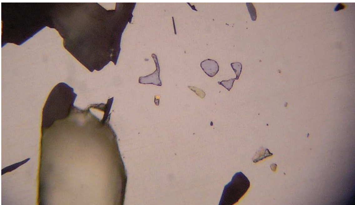
Figure 6. Limited, ultra-fine gold (bright yellow), again associated with galena (pale grey) and chalcopyrite (pale yellow), occluded within euhedral pyrite (beige) within a pyritic variant of the tonalite host at the Two Mile Hill deposit.
