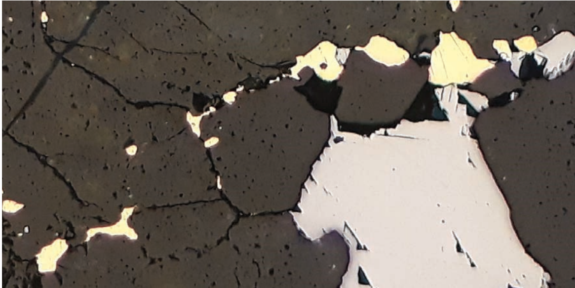
Figure 5. Coarse gold (yellow) associated with galena (pale grey) within quartz veins (dark grey) comprises the vast majority of mineralisation within the Two Mile Hill tonalite deeps deposit.
