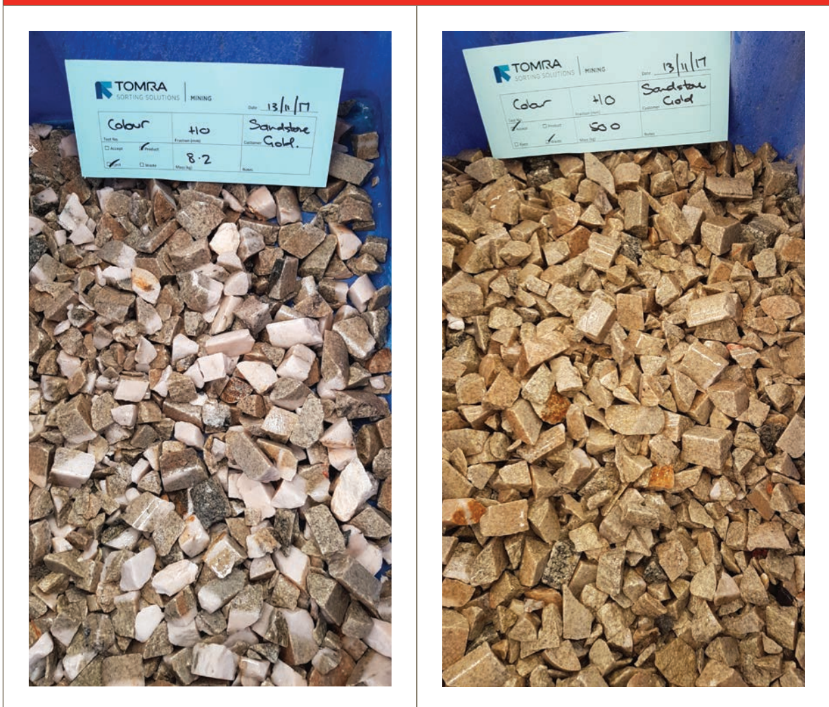
Figure 4. Mineralised quartz (8.2kg) product (left) and waste tonalite - 50kg (right) derived from initial colour ore sorting trial.
