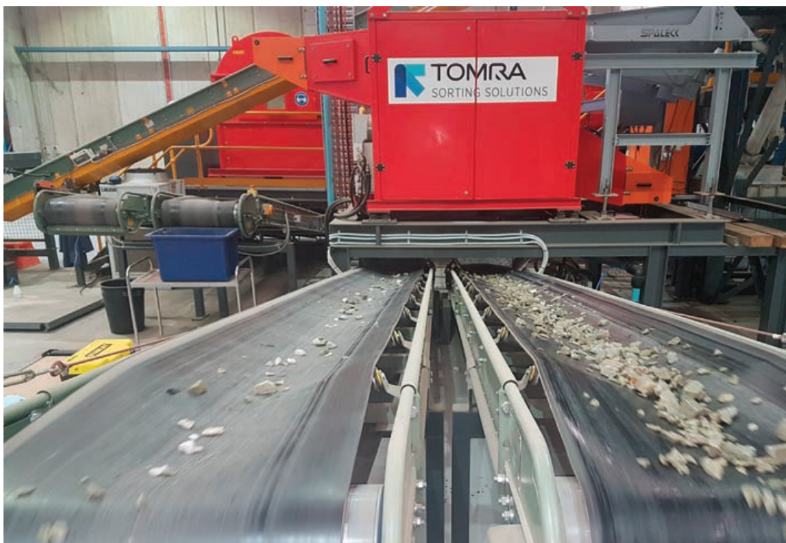
Figure 3. Commercial-scale ore sorting of Two Mile Hill composites at the TOMRA facility in Sydney, with the Colour accepts (predominantly mineralised quartz vein material) belt on the left and rejects (predominantly unmineralised tonalite) on the right.
