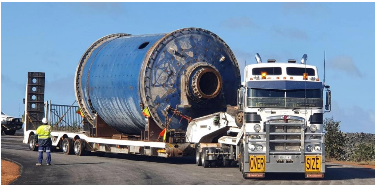
Figure 72: 1.85MW Outokumpu ball mill on the road to Kalgoorlie
