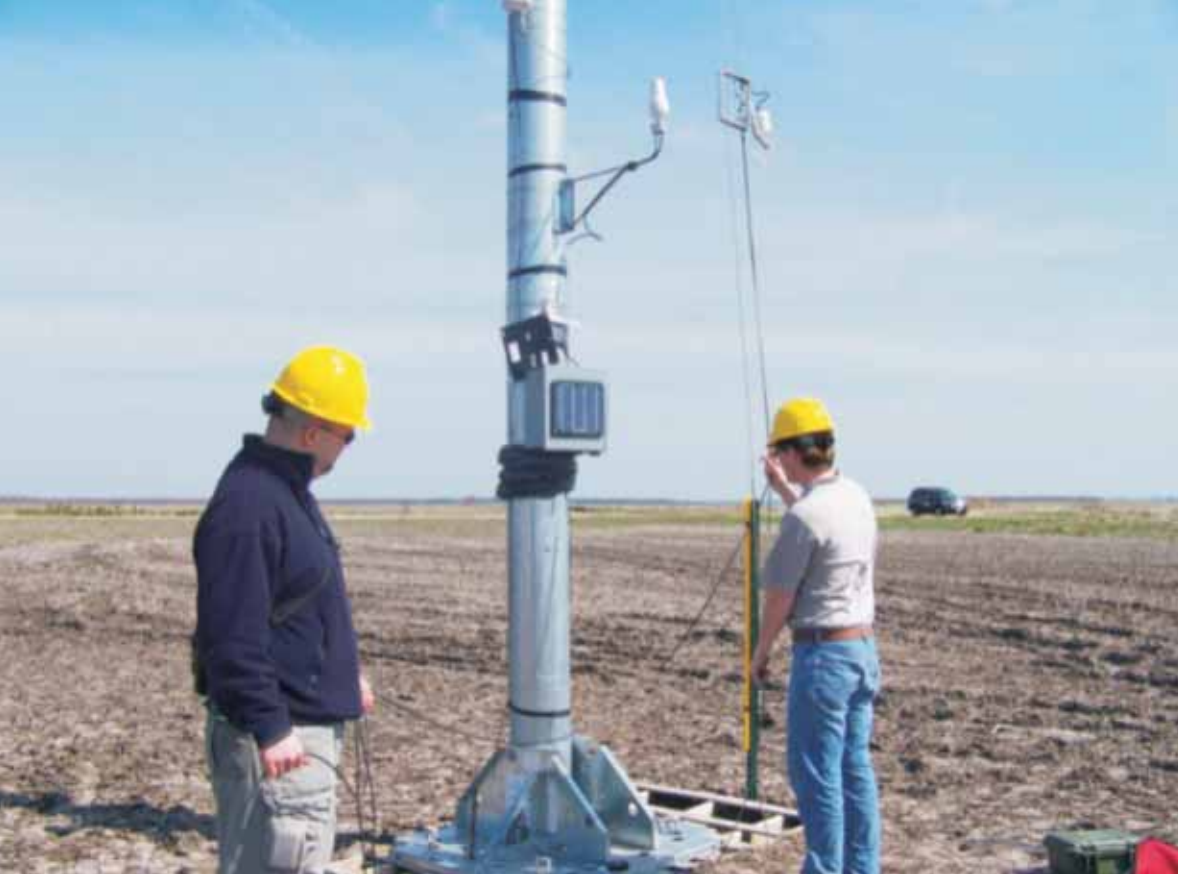
E & E biologists install acoustical bat monitoring equipment to support preconstruction surveys at a proposed wind farm site.
